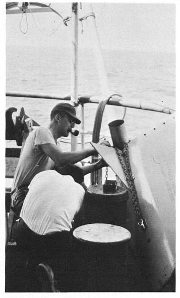
MR. REINERT AND MR. HOLLMON MAKE FINAL CHECKS ON THE FLOW METER FISH
