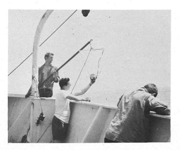
LOWERING A PHOTOELECTRIC CELL TO MEASURE LIGHT PENETRATION IN SEA WATER
